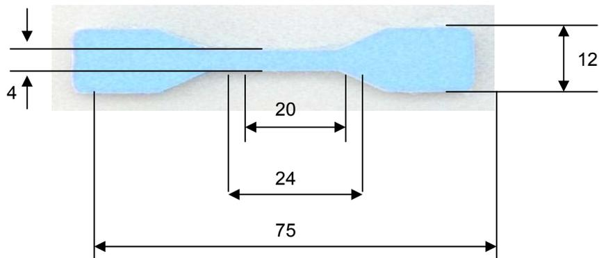
Fig. 4: Test specimen for tensile strength measurement
