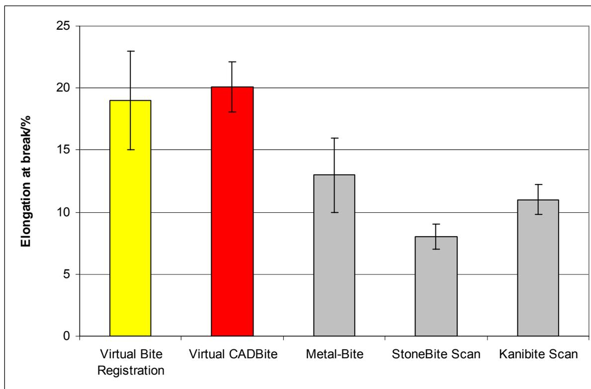
Fig. 6: Elongation at break of different bite registration materials (R&D, Ivoclar Vivadent, 2007)
